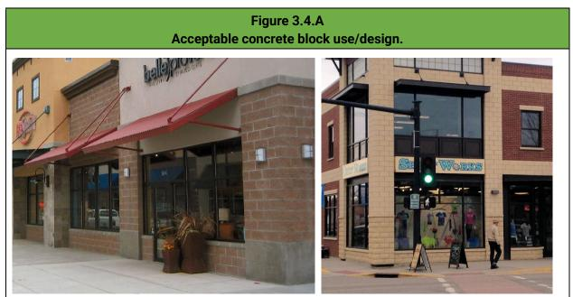
Left: Effective use colored concrete block with trim elements that complements other materials. Right: Colored concrete block with a mix of smooth and textured finish that is well- integrated with other materials.
