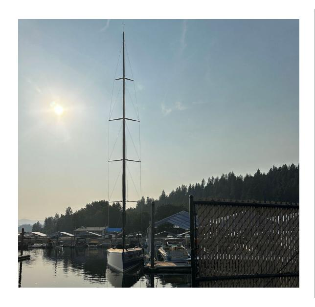
Sizzler, the Idaho Hot Rod 60ft flush-deck speedster – all cold-moulded wood and carbon fiber construction. Designer Tony Castro.
