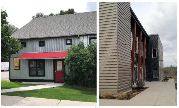
Left: Metal siding with corner and window trim. Note the roof overhang. Right: A good departure example without a roof overhang, but the short length of the walls, amount of window openings, and color/pattern changes create an acceptable design that meets the intent of the standards.
